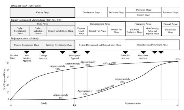
Figure 1. Project life cycle and typical expenditure profile (INCOSE, 2015), added project process in this study by the author
